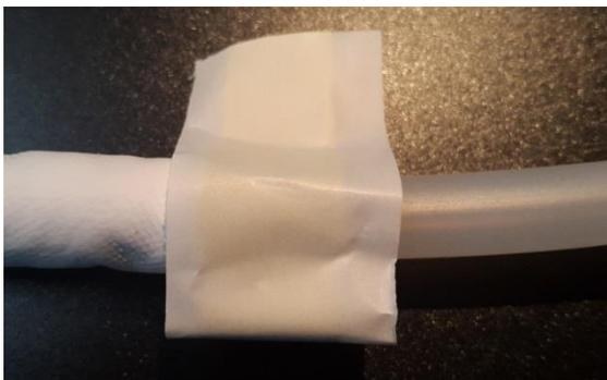
4. Connect the vacuum hose to the vacuum pump. You can incorporate a resin catch container as backup system in between but you will no longer need it.
