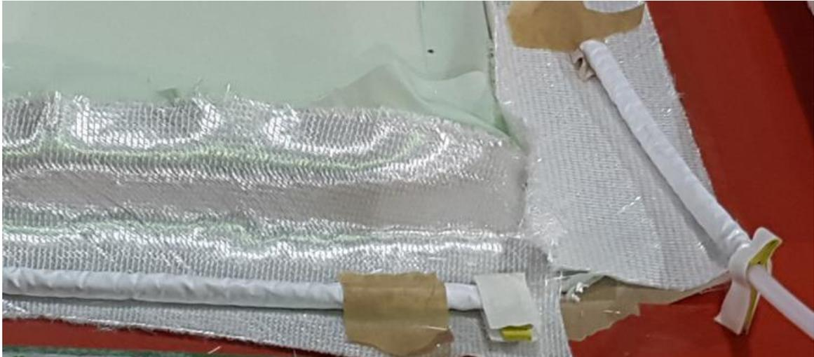
3. To connect the MTI® hose with the vacuum pump we recommend a 3/8" OD solid hose which is plugged into the spiral tube that is inside the MTI® hose. Pull the membrane sleeve over the joint and seal with sealant tape. Be accurate with the sealing operation to prevent resin from entering the vacuum line.
